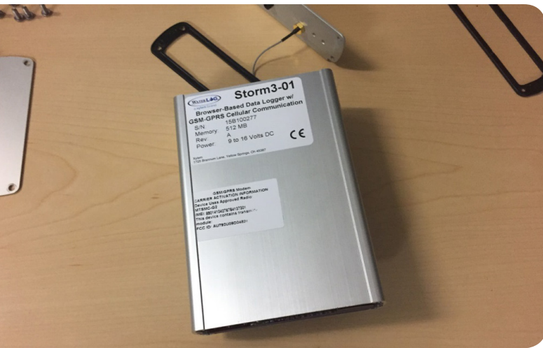
Figure 9: Begin reassembly of Storm 3
