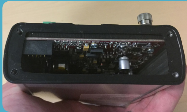
Figure 11: Place the rubber gasket into place
