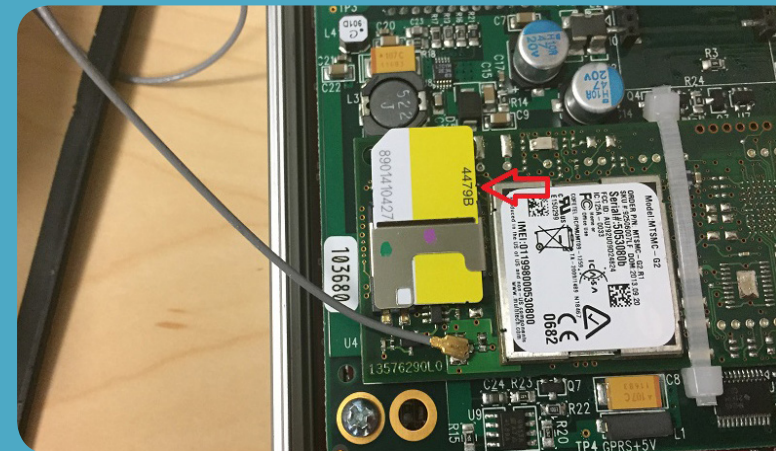
Figure 7: SIM card location on modem board
