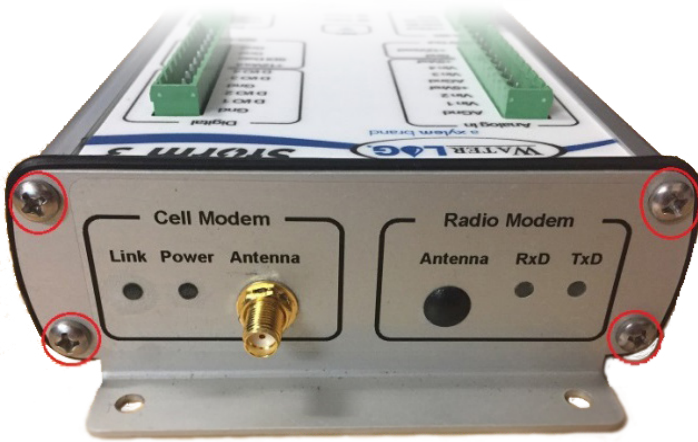
Figure 4: Top plate of the Storm 3 showing the 4 screws
