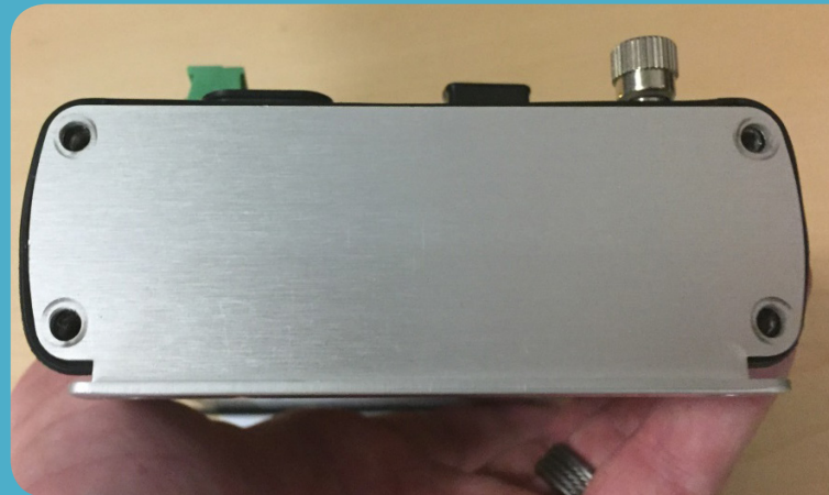
Figure 12: Bottom mounting plate lining up with the holes
