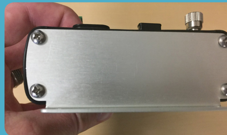
Figure 13: Tighten the 4 screws into place
